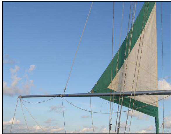
Unfurling the genoa with the pole in place is easy as long as you remember to move the jib lead aft.
