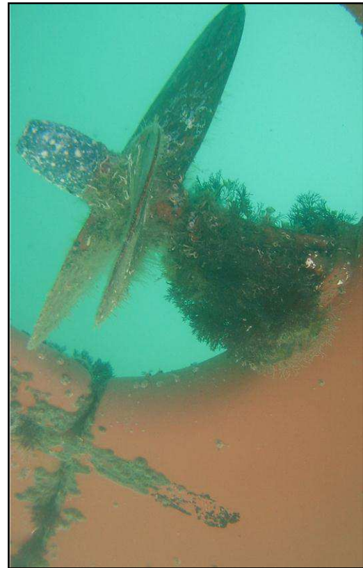
The prop and rudder area has lots of fussy spaces to clean, both to improve performance and to prevent expensive repairs.
