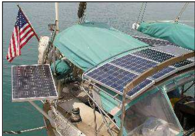
In a sunny climate, our solar panels provide all the power we need. While there is less sun in the winter months, our demand for power is also less as it's not as hot and the refrigerator and fans run less.
