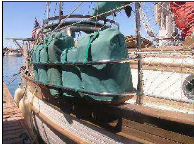
¿Qué Tal? has 4 diesel and 4 gas jerry cans, an extra gas tank for the outboard and a jerry can of water. Port and starboard jerry can racks store them all securely and out of the walkways.
